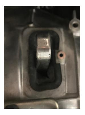
11. Install the braided clutch line, reusing the factory insulative sleeve if possible with some new zipties. Take a second to add a dab of grease to the contact point of the fork adjustment bolt. (Torque spec for the union is 11-12 lb-fts)
