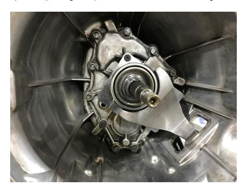
10. Cut a small slit in the old rubber boot that went around the hardline/bleeder and slip it over the fork. It can help to not have the adjustment bolt and jam nut on the fork.
