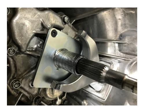
8. Grease the inside of the throw out bearing carrier, you can fully fill the groove with grease. Also add a dab of grease to the bottom of the two 'wings' of the throw out bearing carrier and install the retaining spring for the fork onto the bottom of the carrier.
